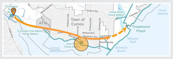
**3c. Gravity Tunnel Alignment – From Lazo Road Hill:** Open cut forcemain to gravity main at Lazo Road with route determined by required slope.
