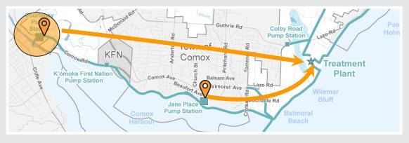
**6. Deep Marine Concept:** Siting forcemain in deep water, connecting existing pump stations to existing treatment and discharge points.
