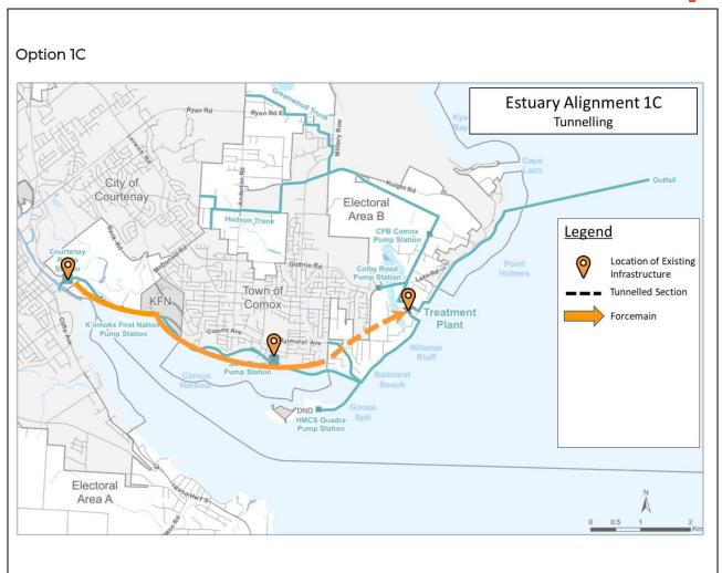
This alignment would involve installation of a new forcemain overland from Courtenay pump station towards the CVWPCC. This forcemain would pass over the Comox Rd. hill. Due to the change in discharge pressure a significant upgrade or rebuild would be required at the Courtenay Pump Station. Several routing options are available including:
