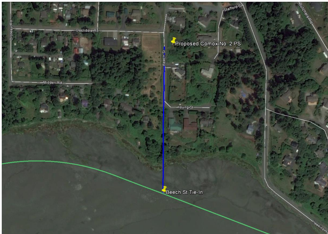
Figure 4-1: Beech Street Tie-In and Alignment (Source: Google Earth)
