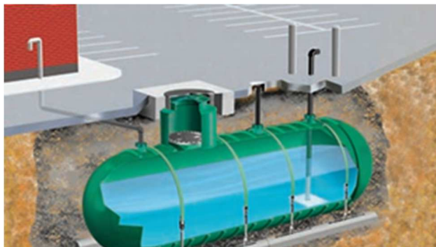
Figure 3 – Example of an underground, fiberglass water storage tanks for fire protection in rural areas
