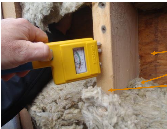
Figure 2.14 Opening 5 Top of wall GL 4/B Moisture Content Readings 30% MC plywood at parapet 35% MC back side of Agepan Damp insulation 22% MC outboard face of stud
