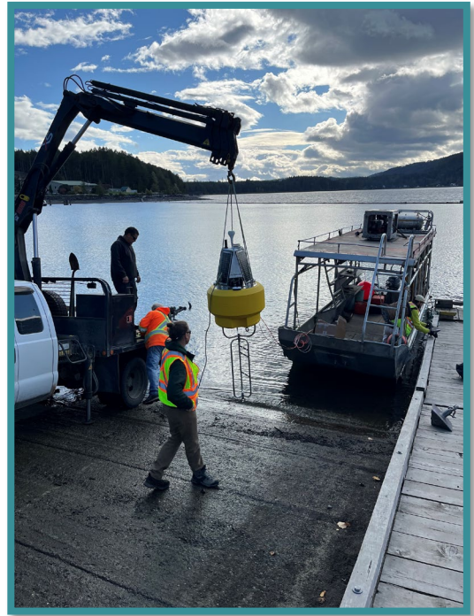
Thermistor buoy deployment on Comox Lake.
